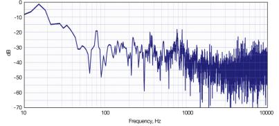
This measurement was taken during a non-optimized, factory floor installation without proper mounting of the SEM-Closure to the floor. Even better performance will be achieved in lab floor and cleanroom floor installations.
